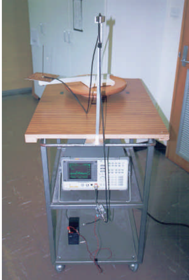
Figure 5-6, Photo of the mobile receiver trolley, showing the rotating antenna on top, spectrum analyser in the middle, and the battery for powering the pre-amp.
